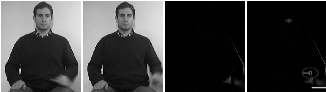
Figure 3.2: The first two pictures show two consecutive frames taken from an example video. The third image shows the difference image of these two frames. The frames are split into two regions, one for the head and one for the hands, and for each of them the difference image is calculated separately. In the last picture, the difference image is presented, but additionally the values of the global motion vectors are drawn into it. There is no visible movement in the head region and therefore only a small light gray circle and a gray ellipsis are shown in the upper half. The light gray line connects the current center of motion (small light gray circle) with the last one and the white bar shows the intensity of motion for the hand region. The gray ellipsis represents the deviation of the motion in x- and y-direction.
