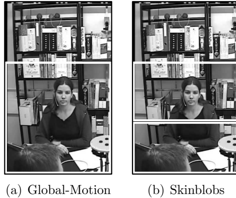
Figure 3.4: Additional to the half images of the left and right camera smaller parts of the images are analyzed. The left image shows the selected region for the additional extraction of global motion features. In the right image two regions for extra skin blob extraction are presented. The upper region is for the detection of the head and the lower one for finding the hands. Only the half frame recorded by the left camera is shown, it also applies to the other half frame and the right camera.
