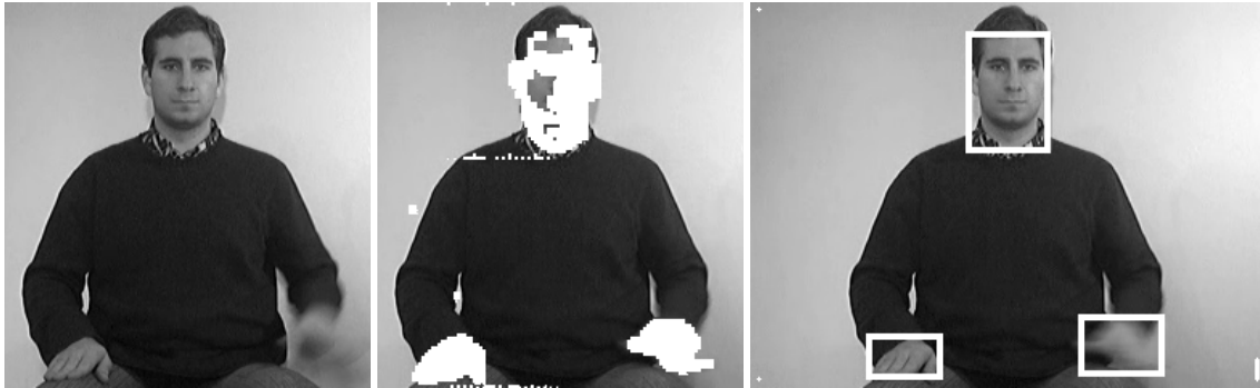
Figure 3.1: The first picture shows a single frame taken from a sample video for illustration of the skin blob detection. In the second picture all detected skin colour pixels are marked by white dots. The frame has been split for the detection task into a head region and a hand region. Especially at the boundaries of the image and of the regions of interest, detection errors are visible. The last image shows the bounding boxes, which are found by the algorithm for the face and the hands. Additionally, the norm of the motion vector for each of these bounding boxes is drawn as a white bar in the corners of the image. The image shows that only the left arm is moved therefore the lower right bar is longer than the other two bars.
