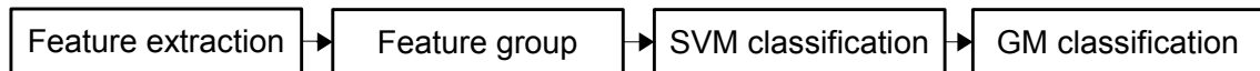
Figure 8.2: Illustration of the combined approach of support vector machines and graphical models. The features and the functionals are extracted and combined to feature groups. These feature groups are classified with support vector machines and the output is used as an input for the classification with graphical models.
