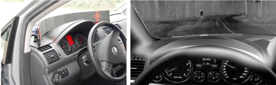
**Figure 3.30:** LED modules for augmenting a Night Vision system. Left: The system displays a simple icon using the LED matrix in the actual line of sight between the driver's head and the obstacle recognized by the NiVi system (image from [Wei+09]). Right: LED line activating a group of LEDs in the line of sight towards the obstacle (image from [Mah+07]).
