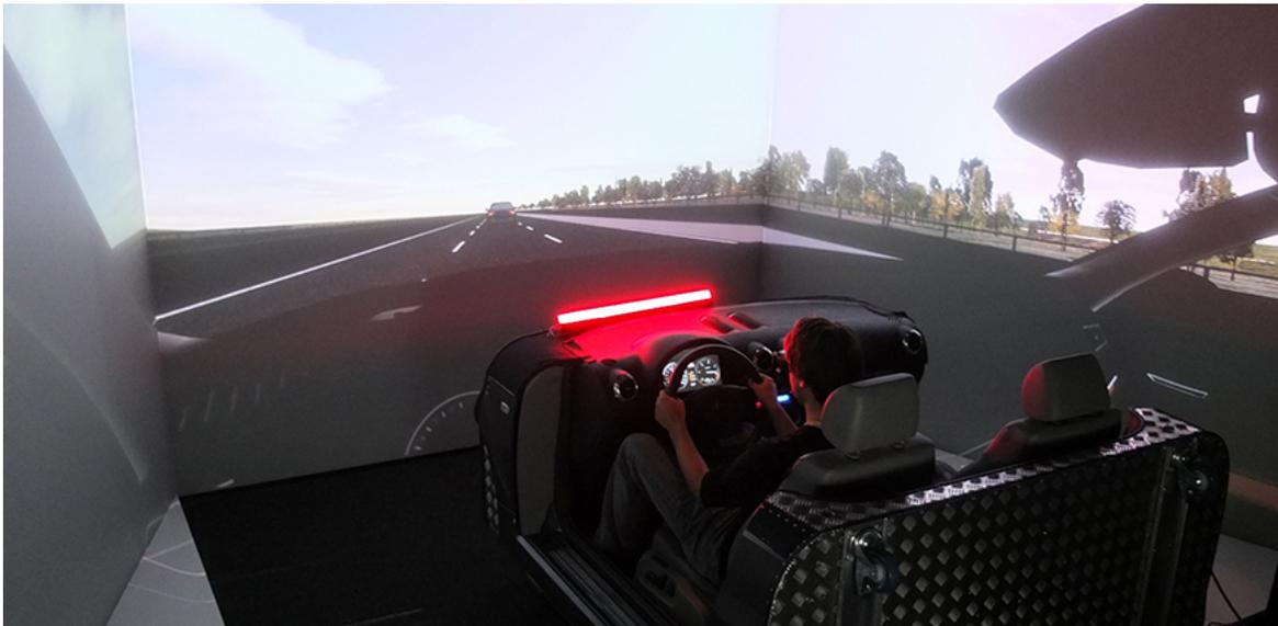
**Figure 6.31:** View of the driving simulator consisting of a real car cockpit with the ISPA LED system and the CAVE for environment projection
