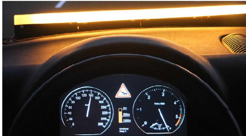
Figure 6.32: ISPA output devices: RGB-LED array on top of the dashboard for encoding distance and proposed deceleration strategy, icon graphics in the instrument cluster depicting the obstacle type and the distance
