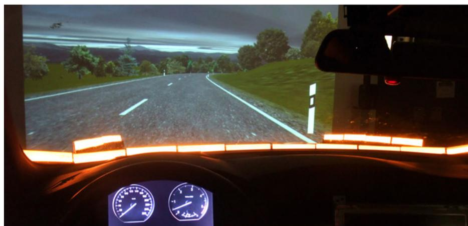
**Figure 3.37:** Driver view of the two LED arrangements on the engine hood. For demonstration purposes all LEDs of both HMI variants are illuminated.
