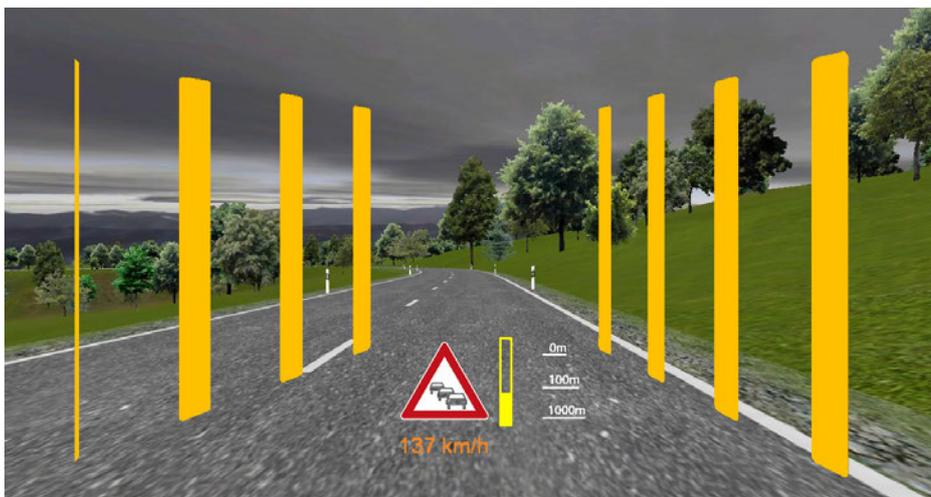
**Figure 3.24:** Picture of the vertical bars produced by the contact analogue Head-Up Display. The bars can be used to alter the speed perception and also the perceived width of the road causing a speed adaption (scene and HUD content digitally mixed).
