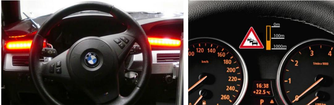
**Figure 3.32:** First LED prototype in combination with instrument cluster visualization. The instrument cluster shows the Iconic HMI, the LED modules are installed left and right of the steering wheel.
