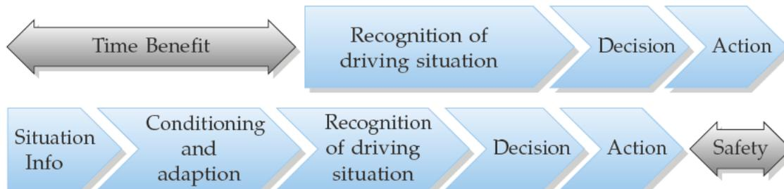
**Figure 3.2:** Safety benefit from earlier driver actions rendered possible through anticipatory ADAS. Timely and detailed information enables a more precise and earlier decision on the needed actions and improves safety (based on [Pop12]).
