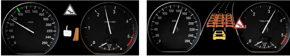
**Figure 3.4:** Initial HMI variants for the anticipatory ADAS: Iconic (left) and Bird's Eye Perspective (right). Both images show the output for exactly the same situation but with very different graphical implementations.
