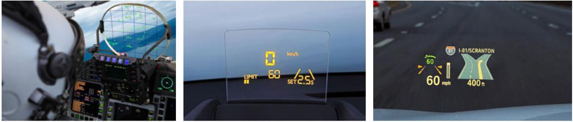
**Figure 3.10:** Implementations of Head-Up displays. First applications were military aircraft (left), later the technology was adopted for cars (center and right picture).
