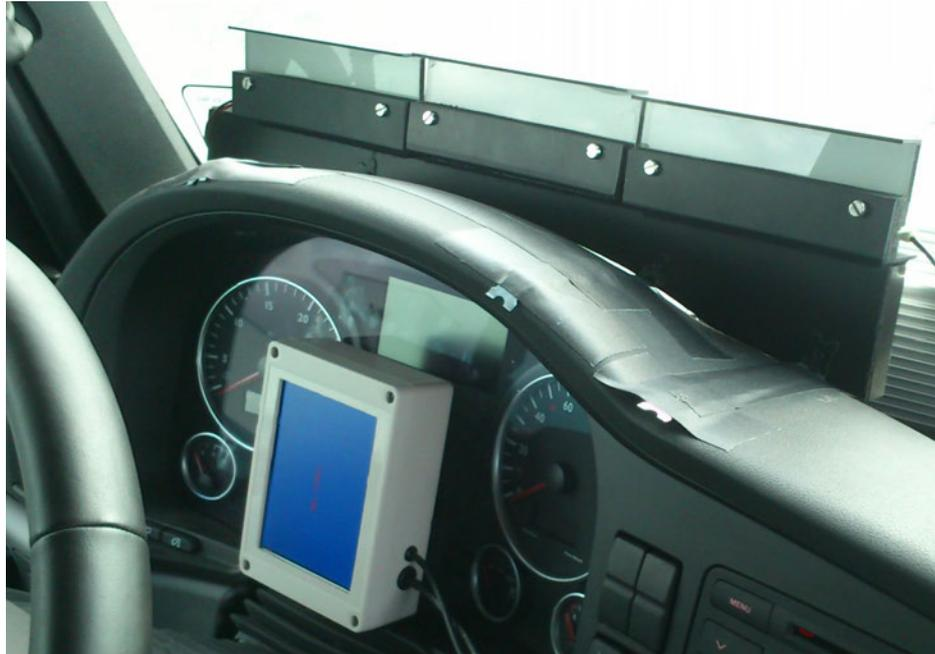
**Figure 4.5:** Picture of the LED modules and the instrument cluster display. The auxiliary display is small enough to maintain a free sight on the built-in instrument gauges.
