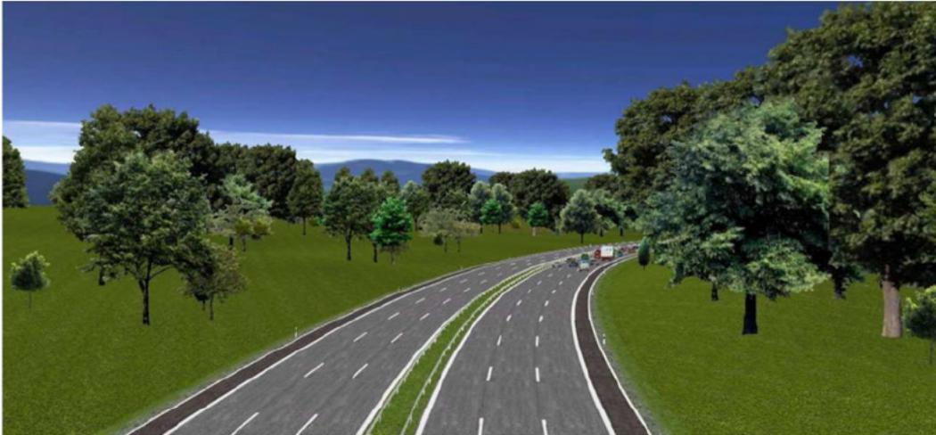
Figure 3.5: View of the situation "Static traffic jam" on a highway. Trees along the road combined with a long-drawn curve make it impossible to see the rear end of the traffic jam in time.
