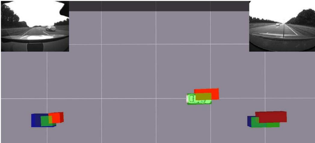
**Figure 2.11:** Matching the object detections of different vehicles for cooperative perception. During an overtaking maneuver each car tracks the others if possible and communicates the positions. Blue boxes represent locally perceived objects, transmitted objects are shown in red. The matching result is marked green (taken from Rauch et al. in [Rau+13]).
