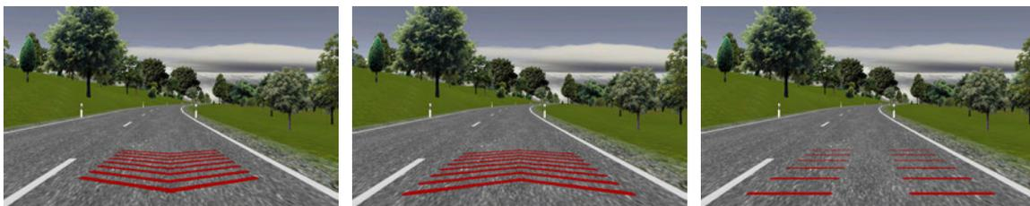
**Figure 3.16:** Virtual road markings in the large Head-Up Display. Different chevron shapes (pointing towards or away from the driver) and transversal bars with different lengths were evaluated in a preliminary experiment (scene and HUD content digitally mixed for illustration purposes).
