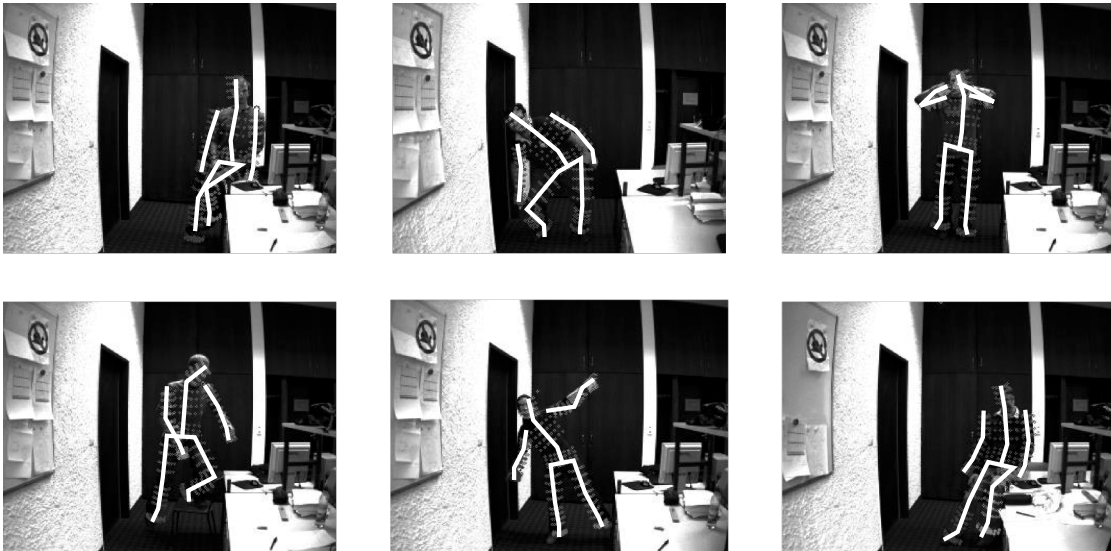
Figure 4.7: Scene from full body tracking. The skeleton was redrawn for better display in monochrome print.
