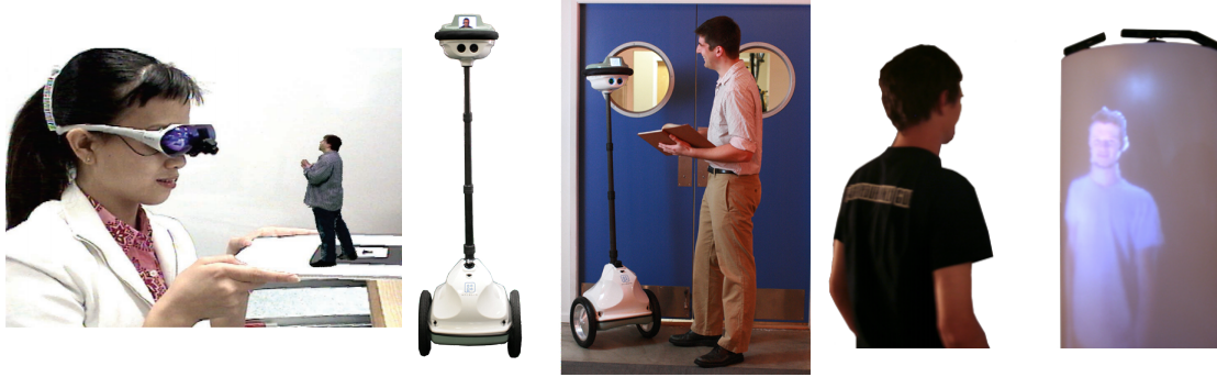
Figure 2.3: Devices used in extended remote collaboration scenarios. From left to right: First AR teleconferencing system by Prince et al. [Pri+02], telepresence robot “QB” by Anybots, TeleHuman by Kim et al. [Kim+12].
