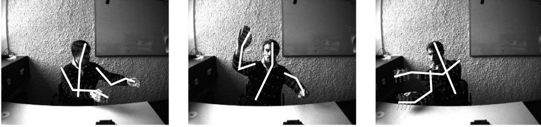
Figure 4.6: Scenes from upper body tracking. The skeleton was redrawn for better display in monochrome print.
