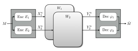
• Independent encoding/decoding:  $C(W_1) + C(W_2)$
