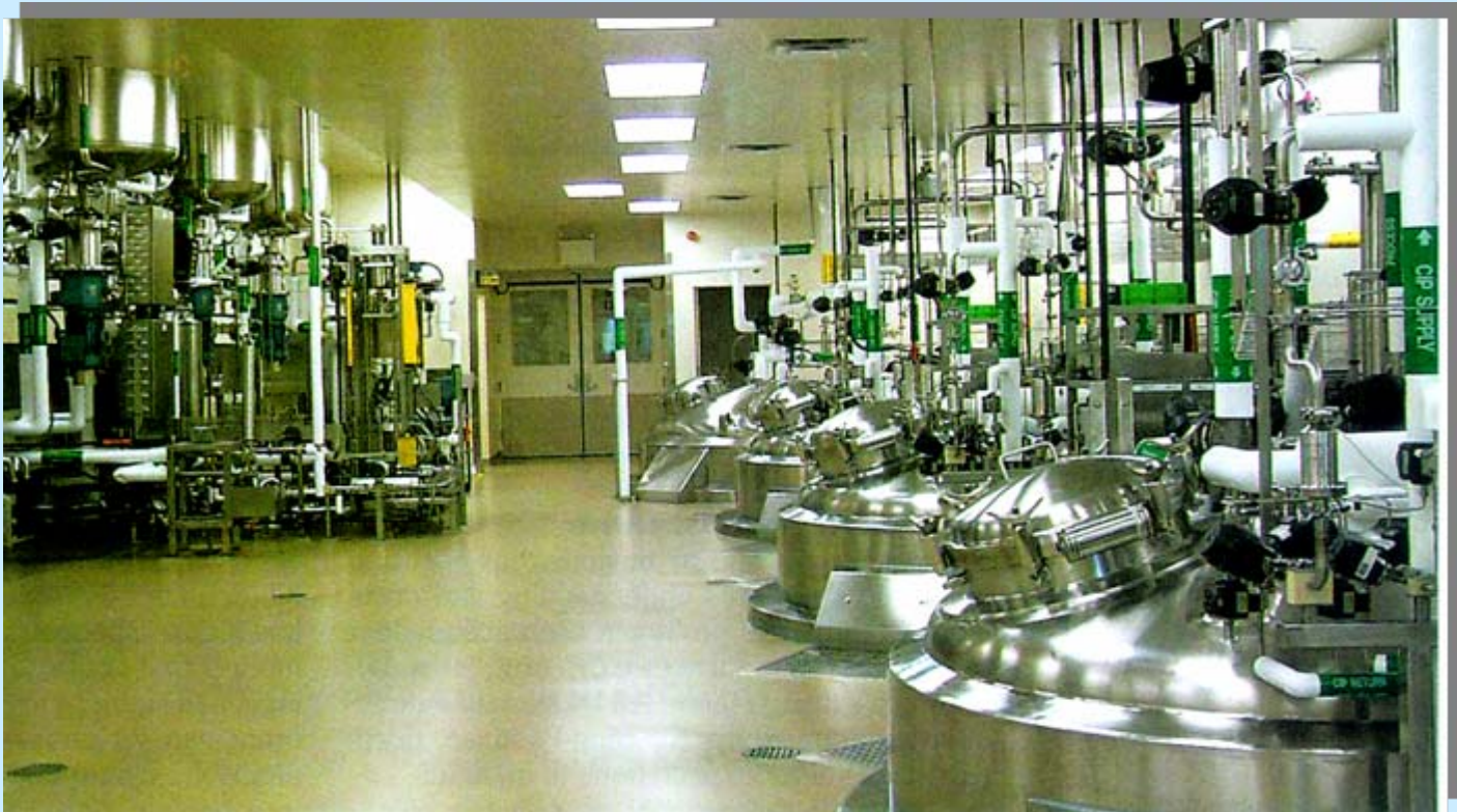
Reactor Line in a Multi-Product, Multi-Stream Batch Process
