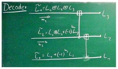
• Replace each polarized bit-channel by a biAWGN surrogate channel with MI matched to  $R_{LM}$  estimated from  $\tilde{L}_i$ , i = 1, 2, 3.
