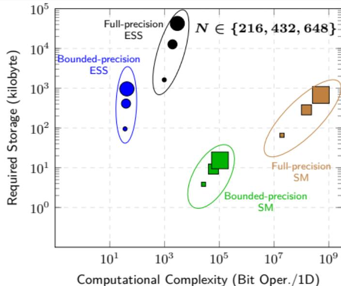
**Solution: Bounded-precision implementation to limit the required storage [6].**
