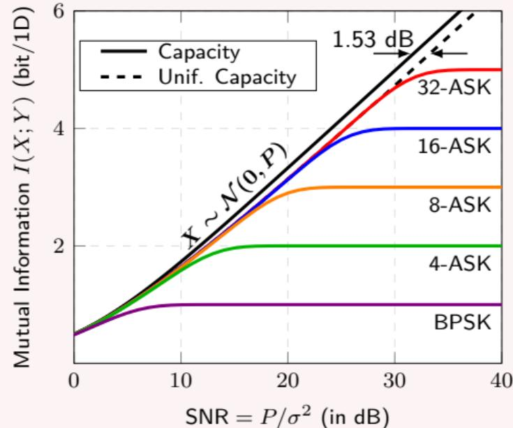
The gap can be closed by transmitting non-uniform (i.e., shaped)  $X$ .
