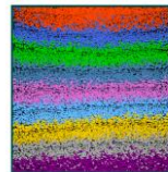
268 Gbit/s LDPC code decoder, area 2.8 mm 2
