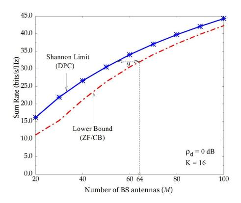
Any sub-optimality can be compensated for with more antennas
