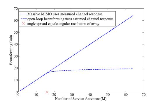
If open-loop beamforming, then not Massive MIMO!
