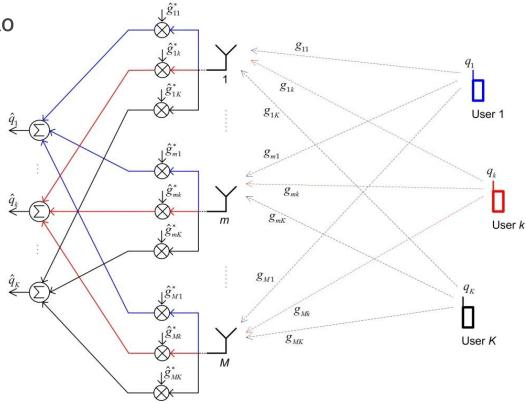
For high SINRs, zero-forcing may outperform conjugate beamforming/matched-filtering
