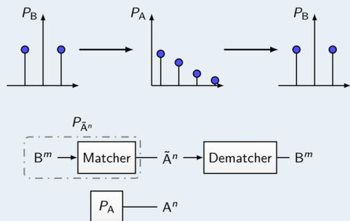
Figure 1: Matching a data block  $B^m = B_1 \dots B_m$  to output symbols  $\tilde{A}^n = \tilde{A}_1 \dots \tilde{A}_n$  and reconstructing the original sequence at the dematcher. The rate is  $\frac{m}{n} \left[ \frac{\text{bits}}{\text{output symbol}} \right]$ . The matcher can be interpreted as emulating a discrete memoryless source  $P_A$ .
