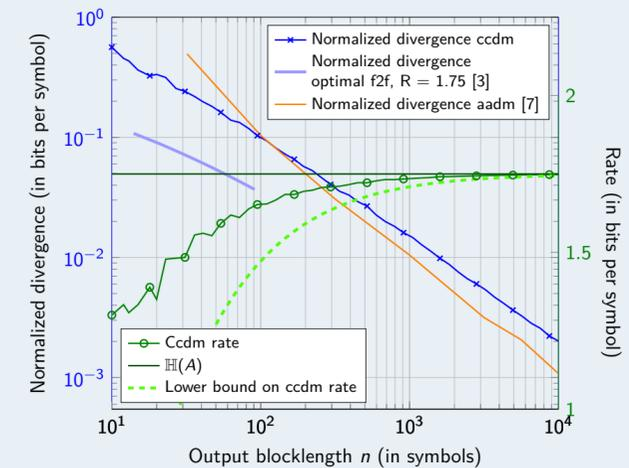
Figure 3: Normalized divergence and rate of ccdm over output blocklength.  $P_A = (0.0722; 0.1654; 0.3209; 0.4415)$ .
