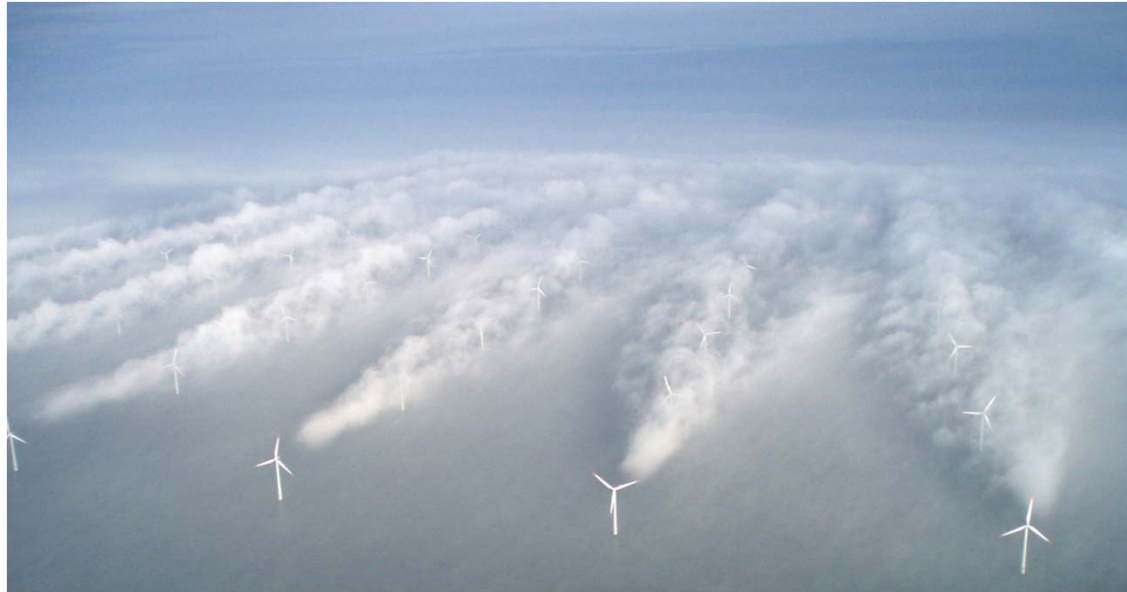
Horns Rev 1 wake effects. Courtesy Christian Steiness
