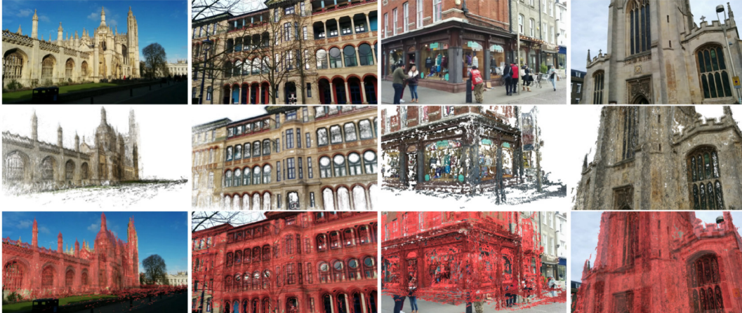
Figure 2.8: The relocalization results for Alex Kendall’s deep convolutional neural network camera pose regressor [45]. Top: input images. Middle: predicted camera poses of the corresponding visual reconstructions. Bottom: input images are shown again with middle images overlaid in red.
