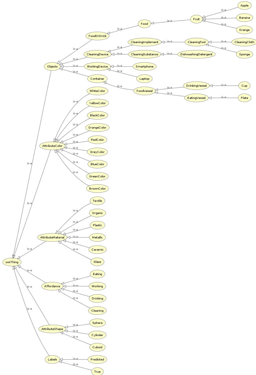
Figure 3.10: OWL Ontology. This tree illustrates the prior knowledge our robot iCub has at the beginning of our experiments. Object properties describe the connections between objects, attributes, and affordance. After learning a new object, the knowledge base is expanded by the new object with its corresponding attributes.
