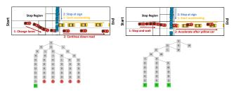
Fig. 2: Comparison of MCTS on a test problem with a stopped car. Letters indicate option being executed: 0 = root, D = default "stay in lane" policy, W = wait, C = Finish/complete level, R = lane change to the right. On the left, we see tree search with a manually defined preference; on the right, we see the tree using the high-level policy acquired through DQN. Green leaves indicate success; red leaves indicate failure. The right side finds a higher-reward solution faster.
