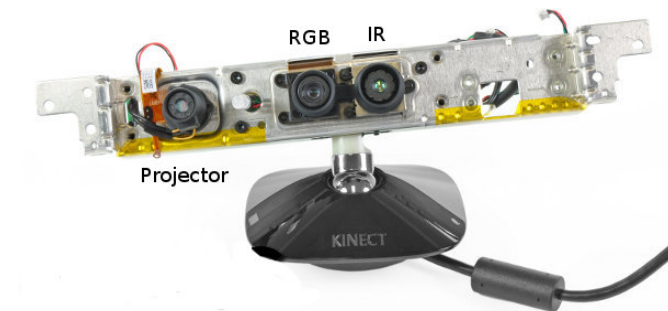
Figure 1: Kinect camera consists of an infrared projector, a RGB camera, and an infrared camera.
