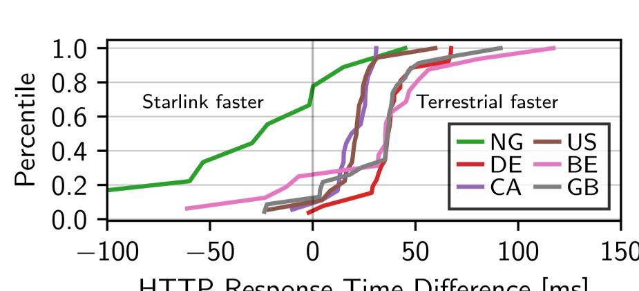
HTTP Response Time Difference [ms] HTTP Response Times are ≈ 20-50 ms higher for Starlink than Terrestrial ISPs
