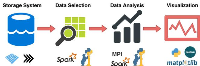
**FIGURE 2.** Prototype of analysis data flow: data is stored in Apache Parquet files (on a NAS-server). Using a Jupyter Notebook, it is loaded and filtered by Apache Spark or pandas and further processed with these tools. There, data mining algorithms are applied and the results are visualized via matplotlib, seaborn, ipyvolum or other frameworks.
