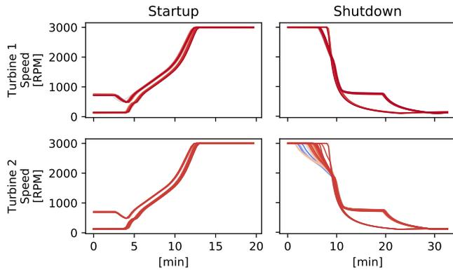
**FIGURE 4.** Visualization of the shaft speed of multiple startup and shutdown sequences for two machines of the same type. All extracted sequences are automatically aligned and plotted on top of each other. While the startups look very similar for both machines, the shutdown process of the second machine is subject to noticeable fluctuations.
