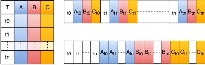
**FIGURE 1.** *Left)* Sensor measurement time series data in tabular form: for each time stamp, there is a value for each signal. *Top-right)* Row-oriented storage. Values are grouped by time stamp. This provides optimal efficiency for writing data to persistent storage. *Bottom-right)* Column-oriented storage. Values are grouped by signal. This is optimal for sequential reading of a single signal.
