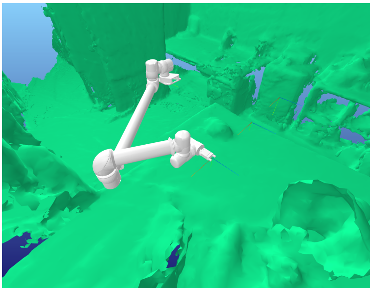
A modular robot solving a CoBRA benchmark in a 3D scanned office.
