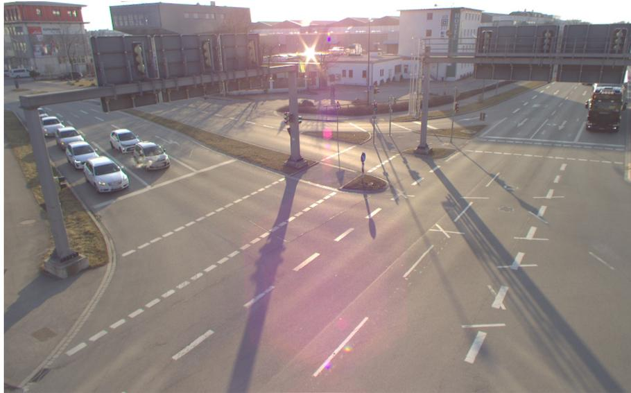
**Figure 6.1:** South2 Basler camera lens flare and reflections.
