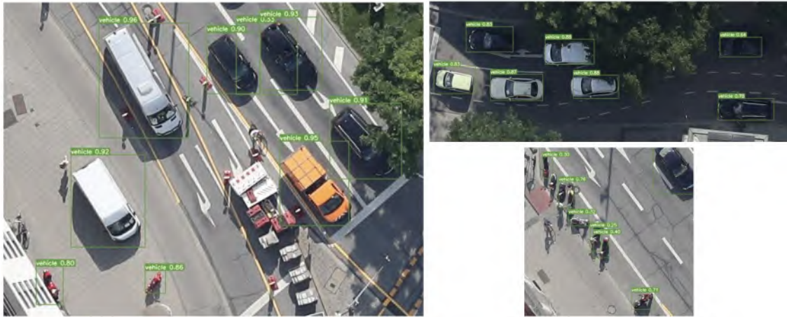
Figure 4.7: YOLOv7 inference result, with 2560 X 2560 image-size parameter value, on an image of the 2021-07-21-ATM_43 sequence.
