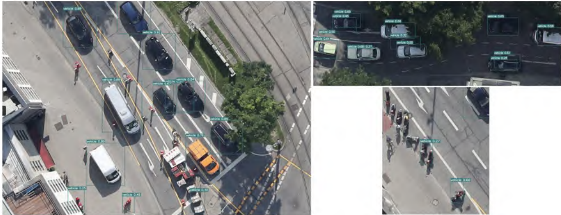
Figure 4.3: YOLOv7 inference result, with 640 X 640 image-size parameter value, on an image of the 2021-07-21-ATM_43 sequence.
