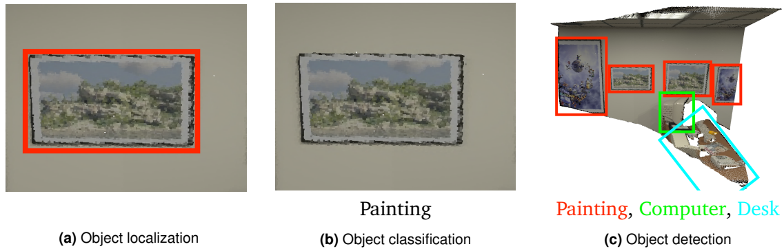
Figure 2.4: Distinction between three computer vision task in a point cloud using 2D bounding boxes [140].
