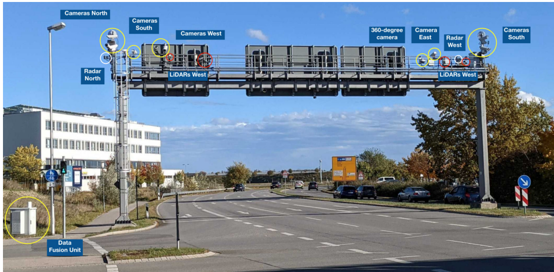
Figure 2.1: Overview of sensors placed on the s110 sensor station in Garching-Hochbrück
