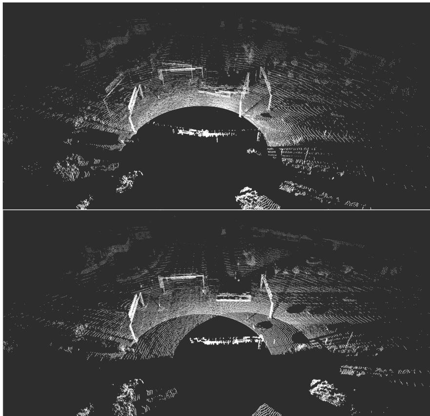
**Figure 3.14: Point cloud registration results.** Up: unregistered point clouds. Down: corresponding registered point clouds.
