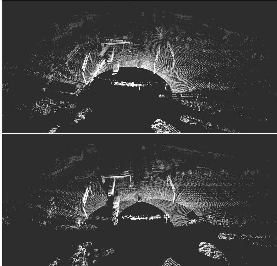
**Figure 3.13:** Up: unregistered point clouds. Down: corresponding registered point clouds.
