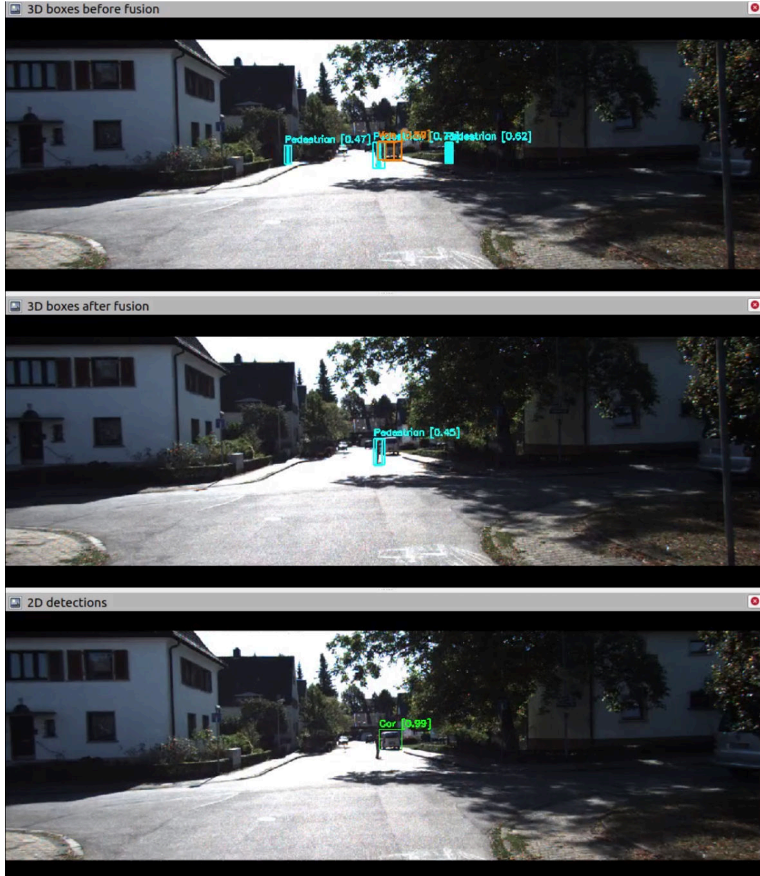
Figure A.17.: This an example of a situation where the LiDAR-based detection is of advantage when bad light conditions are against the 2D detection. YOLOv4 misses to identify the pedestrian in the shadow standing in the middle of the street, but CenterPoint both before and after fusion does detect this pedestrian very well
