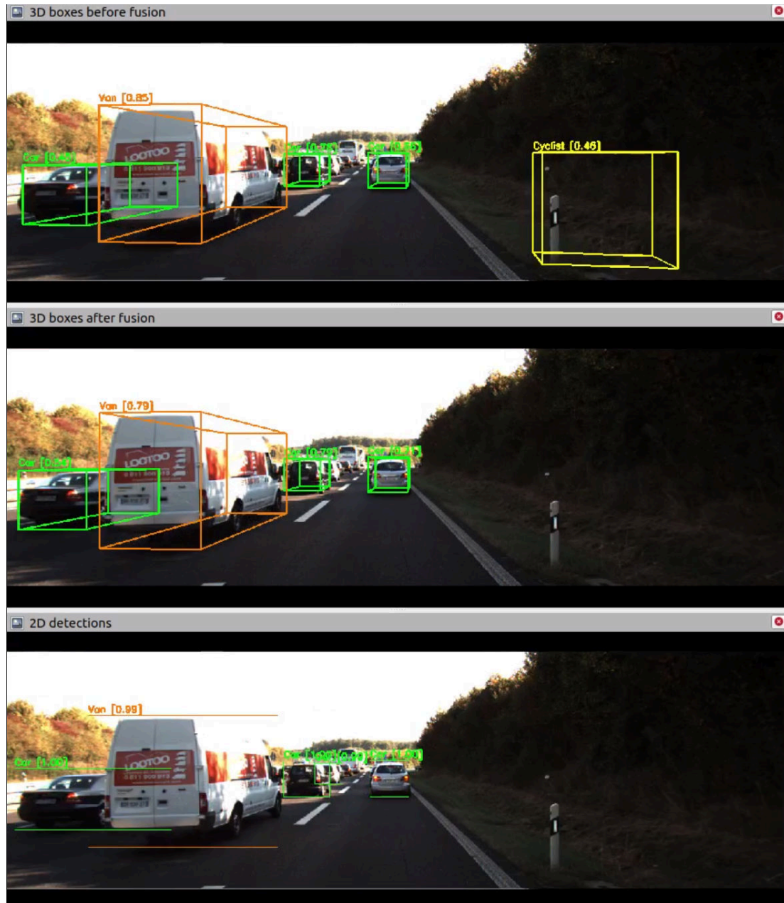
Figure A.8.: A FP cyclist confused with a pole on the highway was removed after fusion on the right side of the scene
