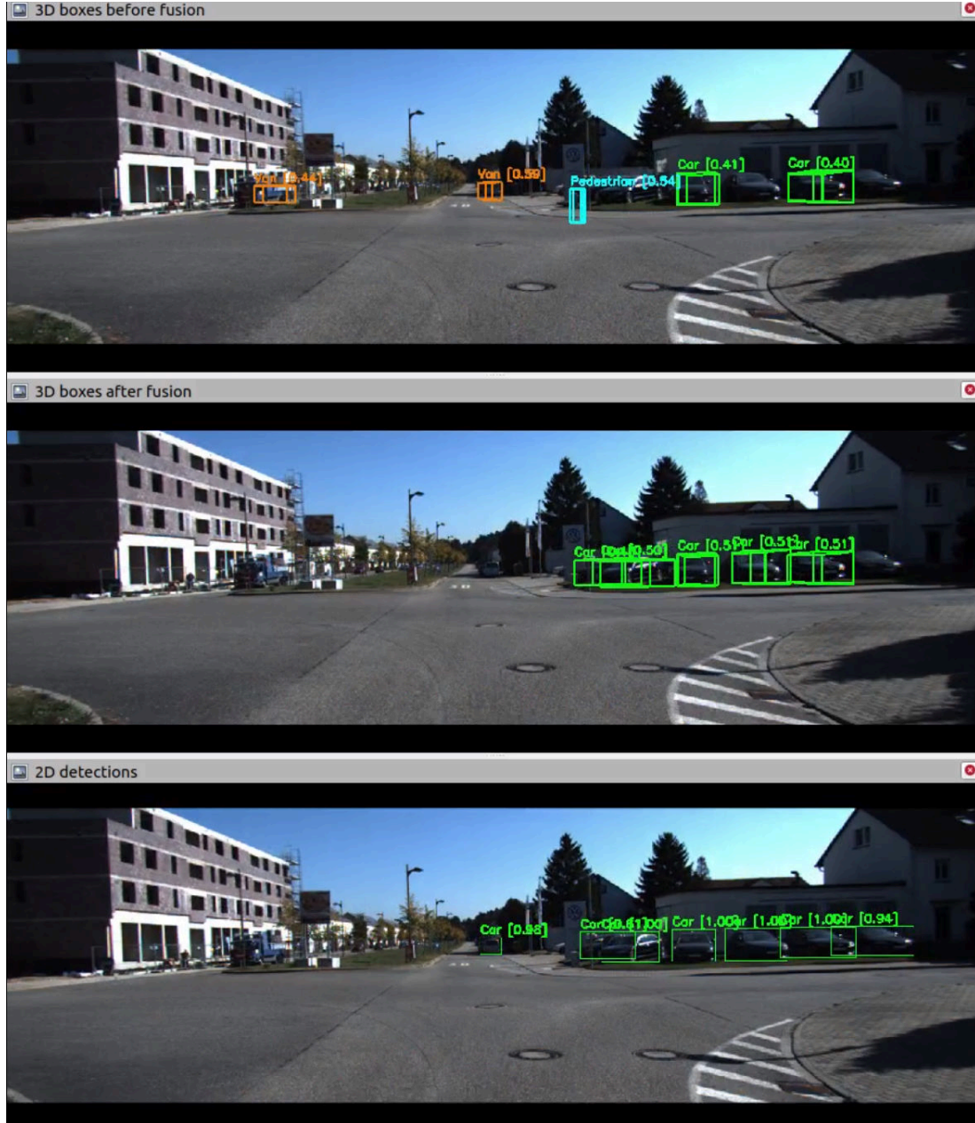
Figure A.5.: The 2D detections from YOLOv4 enabled the detection of more 3D car boxes, (only 2 before vs 6 after fusion) plus some other FPs were removed
