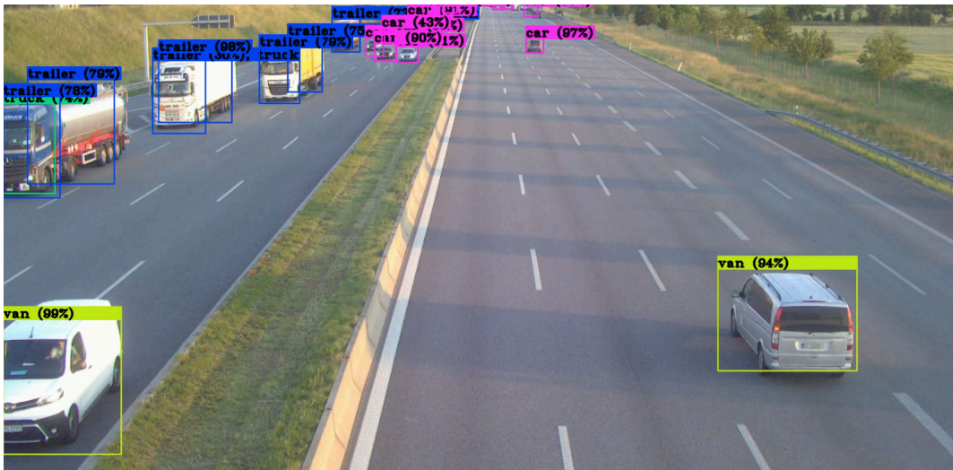
Figure 5.11.: 2D boxes predicted by YOLOv4 on an image from the highway A9 that is a portion of the testbed in Providentia++ , where the classes 'Car', 'Van', 'Truck' and 'Trailer' are detected
