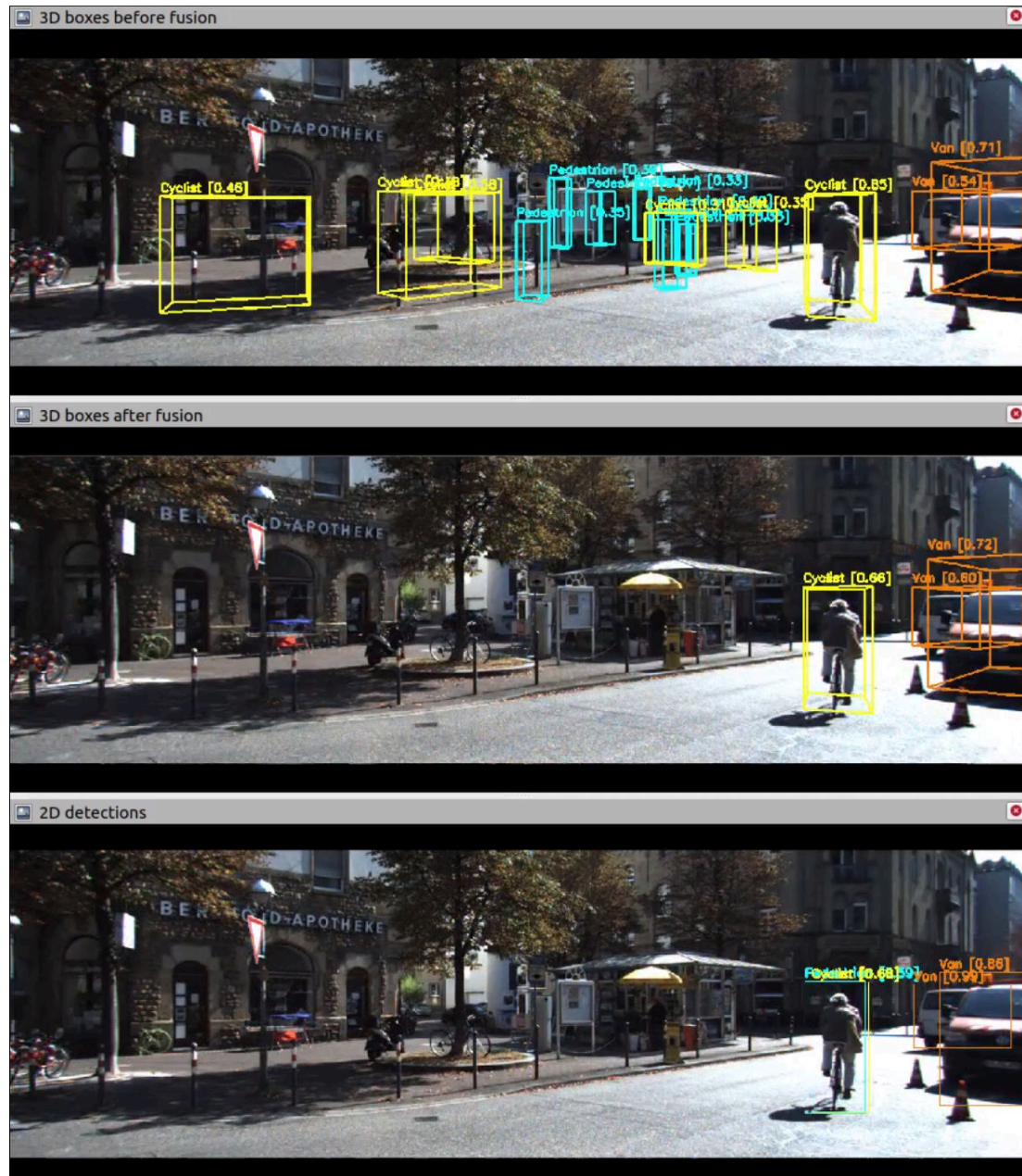
Figure 5.3.: A significant amount of cyclists and pedestrians FPs are removed from the scene after fusion
