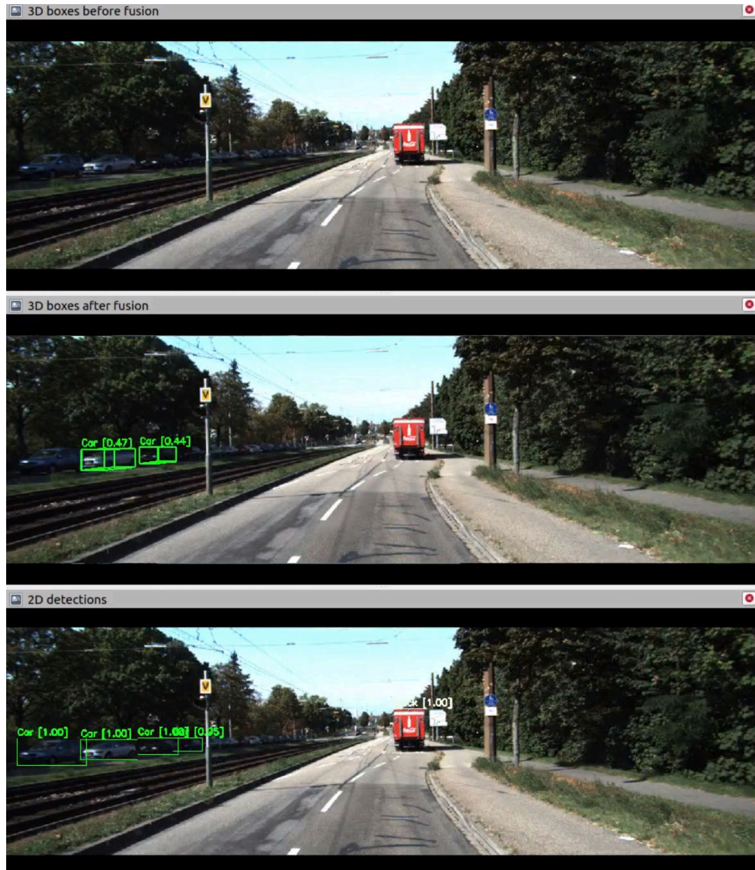
Figure A.4.: The detections in 2D helped to increase the recall to locate two cars on the left that were missed previously
