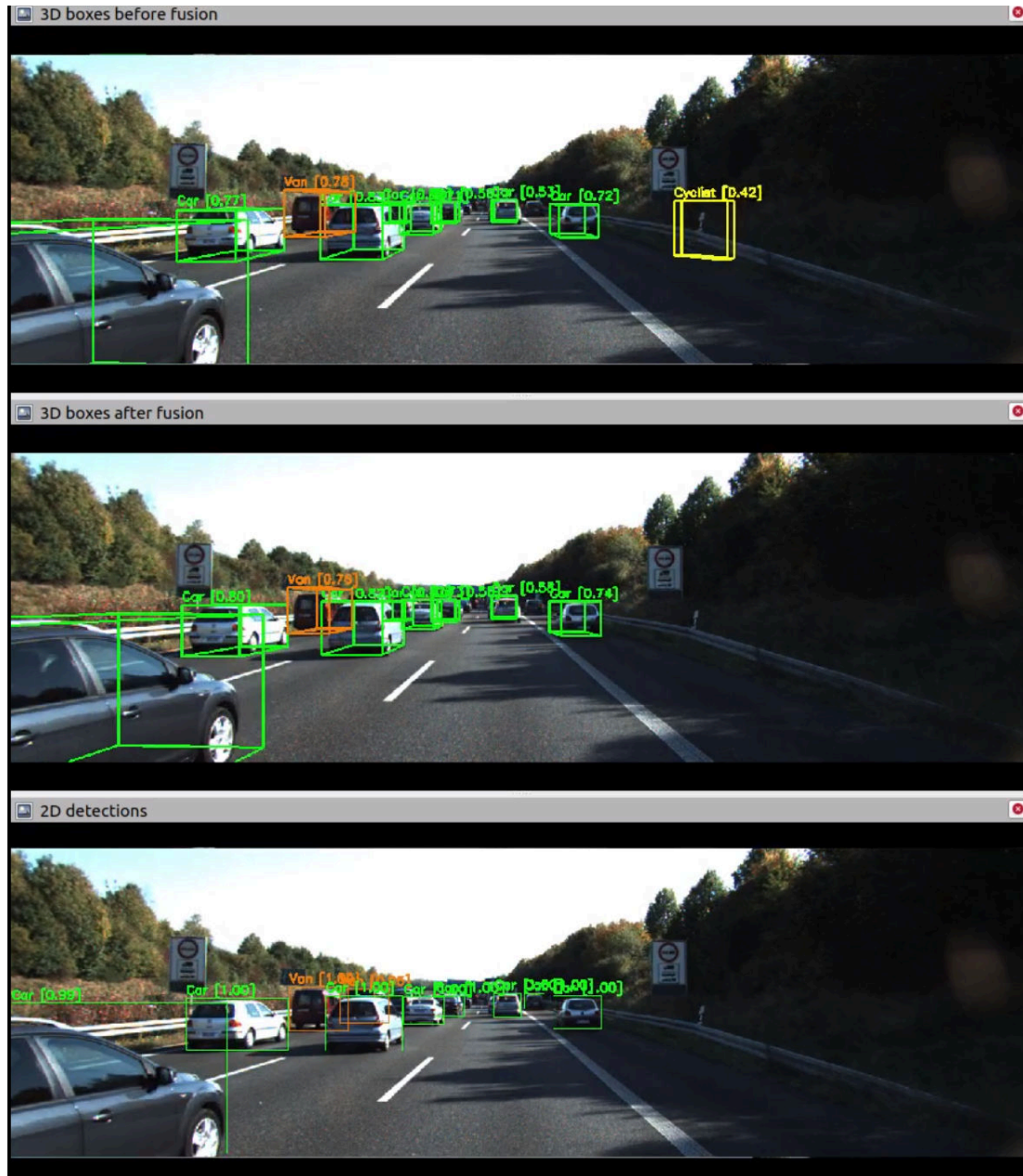
Figure A.7.: A FP cyclist confused with the highway barrier was removed after fusion on the right side of the scene
