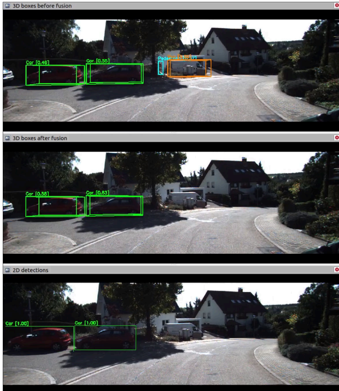
Figure 5.6.: The 3D box of the TP van in the middle predicted by CenterPoint , was suppressed after fusion because YOLOv4 failed to detect it
