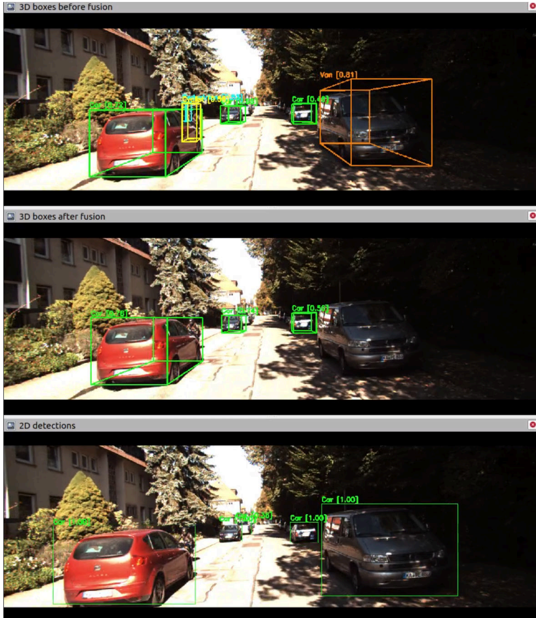
Figure A.10.: The gray big vehicle on the right was well detected by both CenterPoint and YOLOv4 , but there is a strong disagreement between the predicted labels that causes the 3D box 'Van' to be removed after fusion
