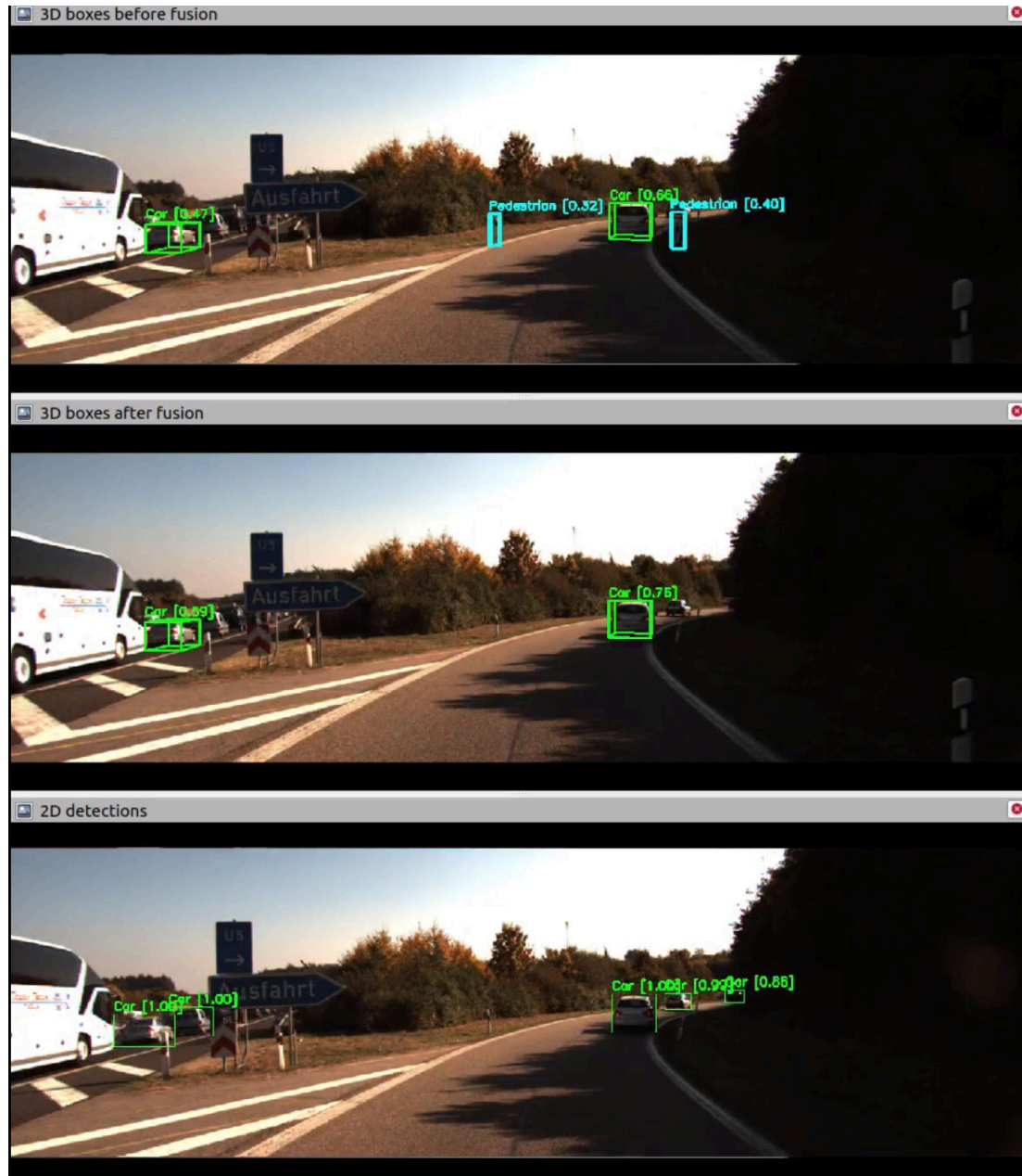
Figure A.3.: The fusion method deletes FPs pedestrians confused with poles on the road boundaries
