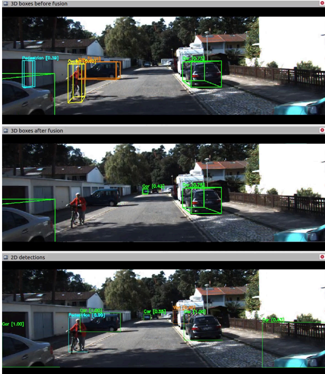
Figure A.11.: A FP pedestrian was deleted on the left side of the street after fusion, but also the TPs 'Cyclist' and 'Van' were suppressed because YOLOv4 detected these with different labels 'Pedestrian' and 'Car' respectively. Also after fusion a car in the middle of the scene in the far range got detected in 3D thanks to a corresponding 2D 'Car' match from YOLOv4
