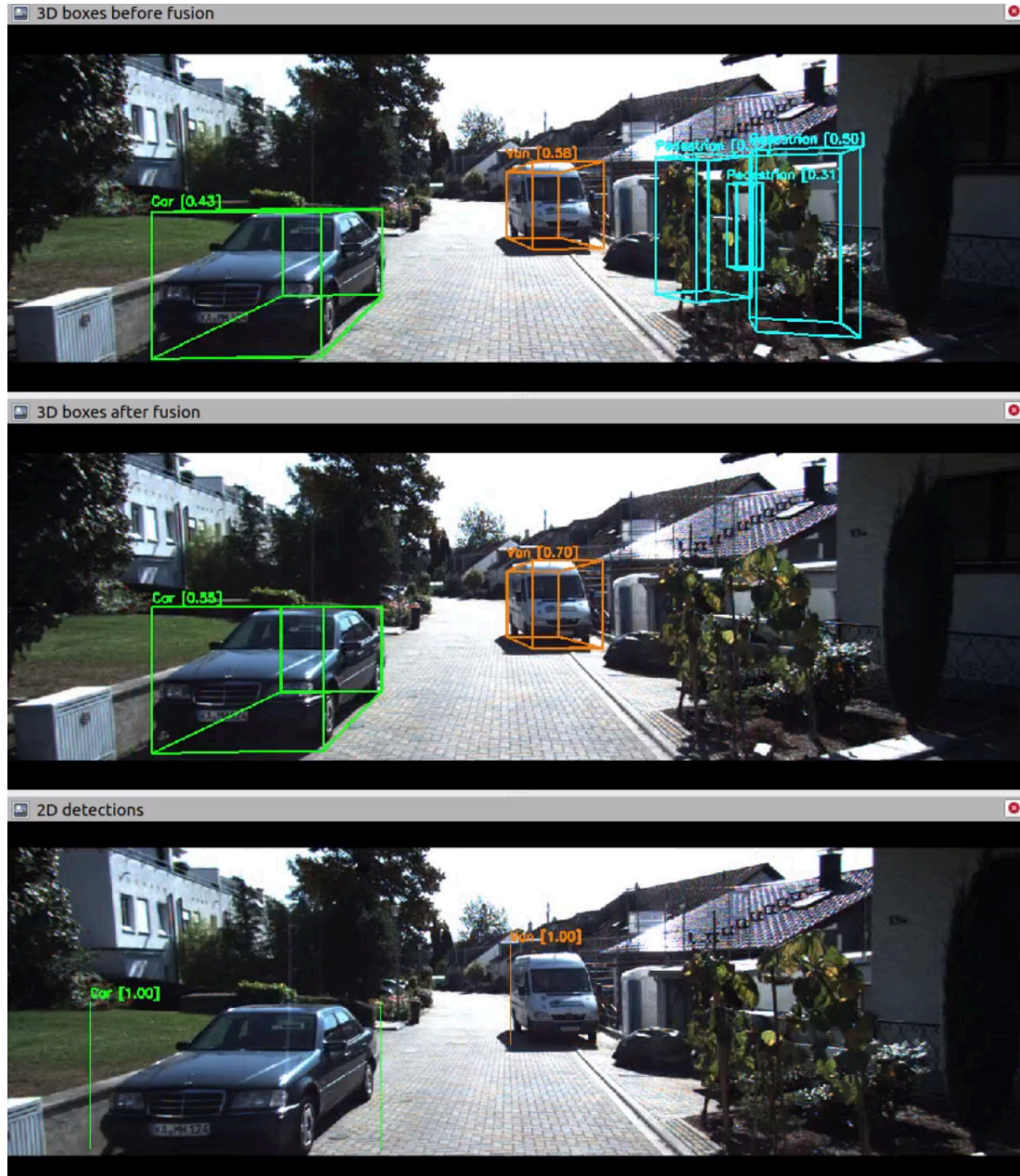
Figure 5.5.: Fusion enhances the confidence scores of the predicted objects, CenterPoint alone estimates 'Car' [0.43], 'Van' [0.58]. CLOCs boosted the scores to be 'Car' [0.55], 'Van' [0.70] and deleted the false pedestrians on the right confused with plants before fusion
