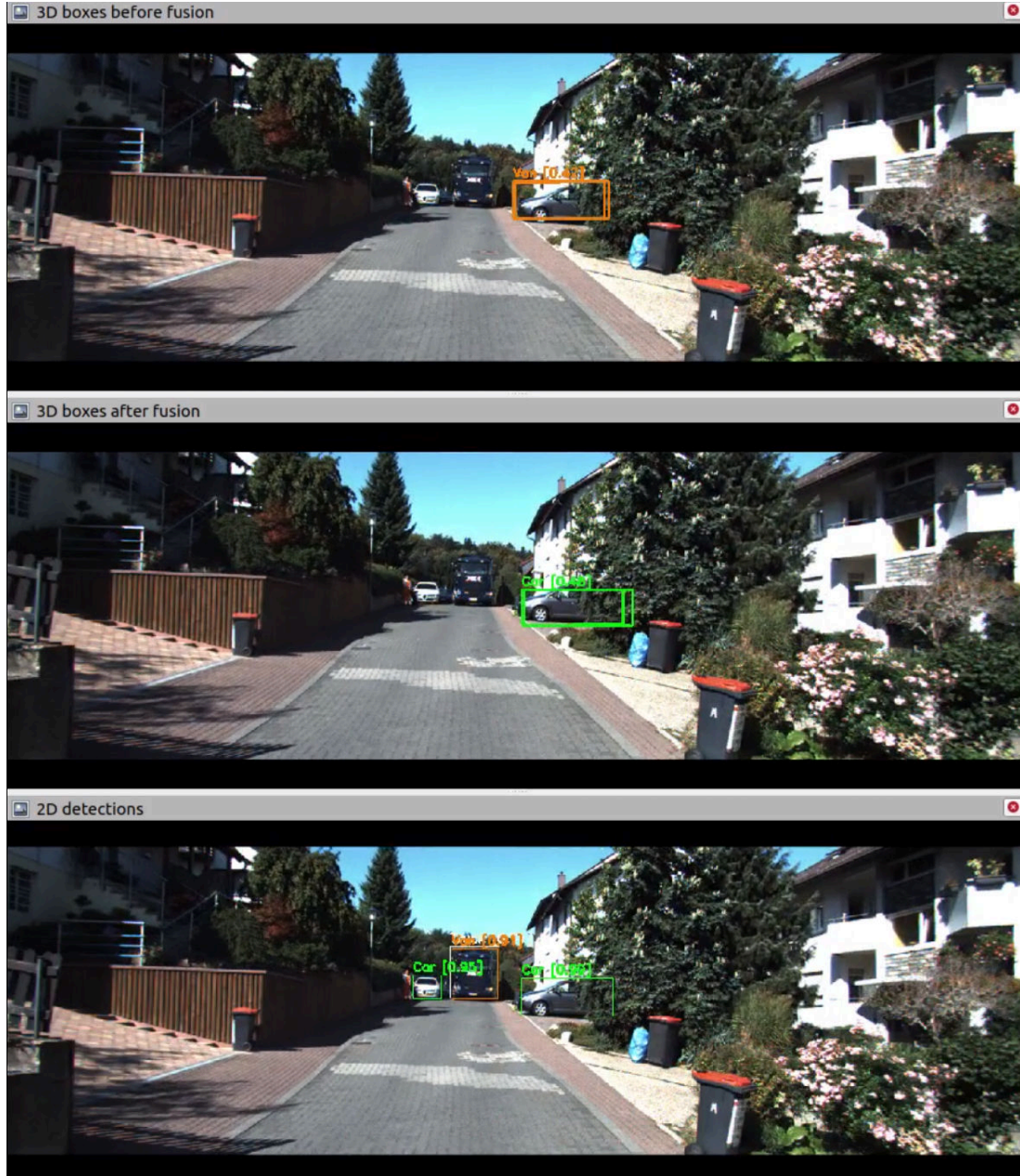
Figure A.1.: The predicted 3D box as 'Van' is corrected after fusion with CLOCs thanks to the right classification in 2D. YOLOv4 additionally detects a car on the left in the far range that the 3D detector was not able to locate
