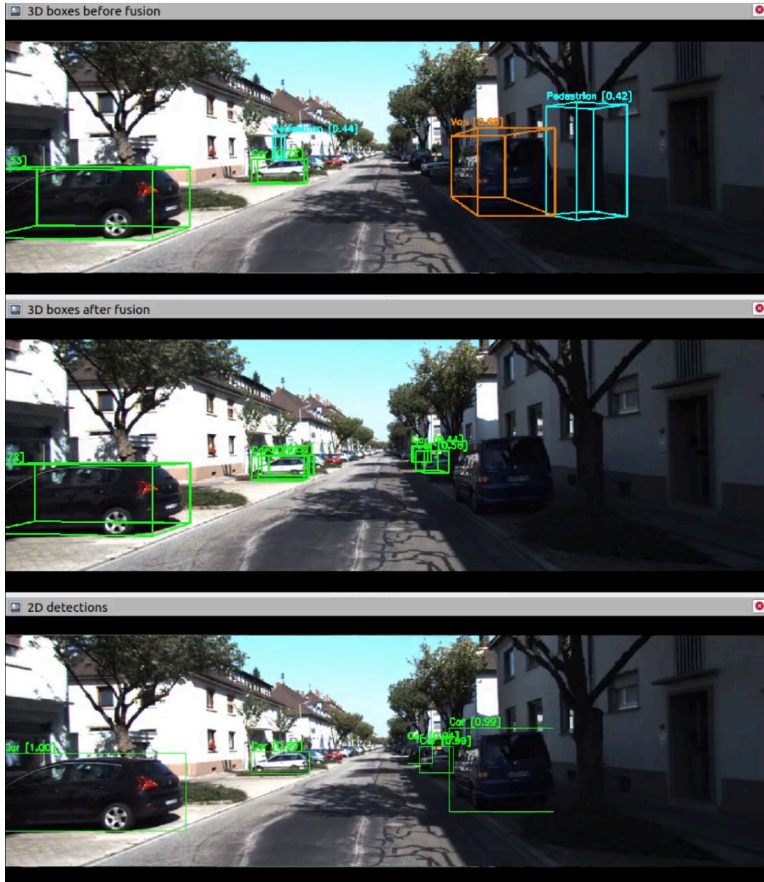
Figure A.12.: A FP pedestrian confused with a tree trunk was removed and more cars on the right side of the street got detected after fusion, but also the TP van was deleted since YOLOv4 predicted this van to be a car instead
