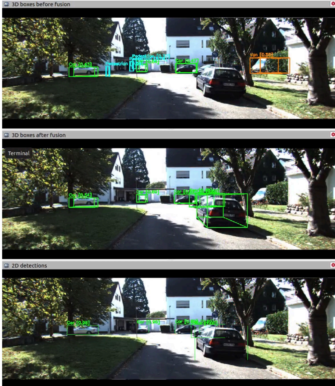
Figure A.9.: The white vehicle on the right was correctly detected as 'Van' by CenterPoint , but after fusion the TP was removed since a detection in 2D from YOLOv4 was missing, so CLOCs considered the initial TP as a FP
