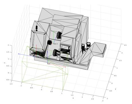
A machine tending task with possible placements for the robot's base within the green box.
