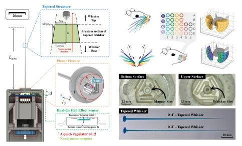
A). The basic structure for our magnetically transduced tapered whisker sensor with details B). The array of an average rat is organized in rows and columns with specific pattern and different dimensions for each single whisker.
