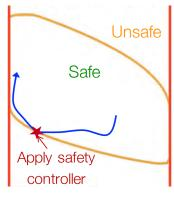
If the RL algorithm makes the agent leave the safe set, a safety controller is applied to keep the system inside the safe set (figure taken from: Melanie N. Zeilinger *Towards Safe Learing-Based Control*, around 2014).
