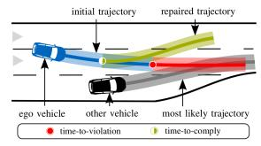
Sketch of TC. The initially-planned trajectory for the ego vehicle violates the traffic rule starting from time-to-violation (TV) since it does not yield to vehicles entering the main carriageway from the access ramp. In our approach, the vehicle should take action before TC to avoid the incompliance.
