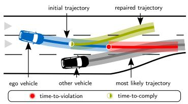
Sketch of trajectory repairing regarding traffic rule violations. The initially-planned trajectory for the ego vehicle violates the traffic rule since it does not yield to vehicles entering the main carriageway from the access ramp [3].
