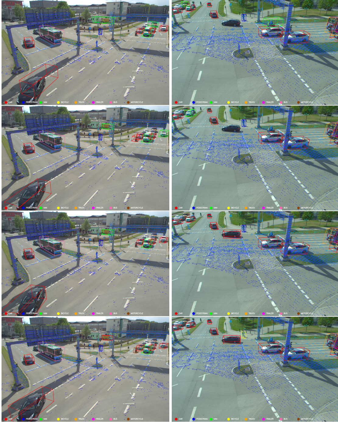
Figure 5.15: The figure shows the detection results of the PV-RCNN model on the same point cloud frame at different stages in the active training process, employing the tCRB strategy. The first row corresponds to the detections of the model's state at epoch 130 (the 6th selection cycle). The second row corresponds to epoch 150 (the 7th selection cycle). The third row corresponds to epoch 170 (the 8th selection cycle), and finally, the last row corresponds to epoch 190 (the 9th selection cycle).
