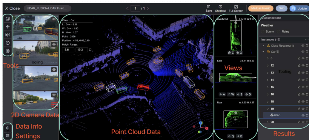
Figure 3.11: The Xtreme1 annotation tool main interface with intuitive tools for labeling objects, combining camera images and 3D views to help users annotate and track multiple objects.
