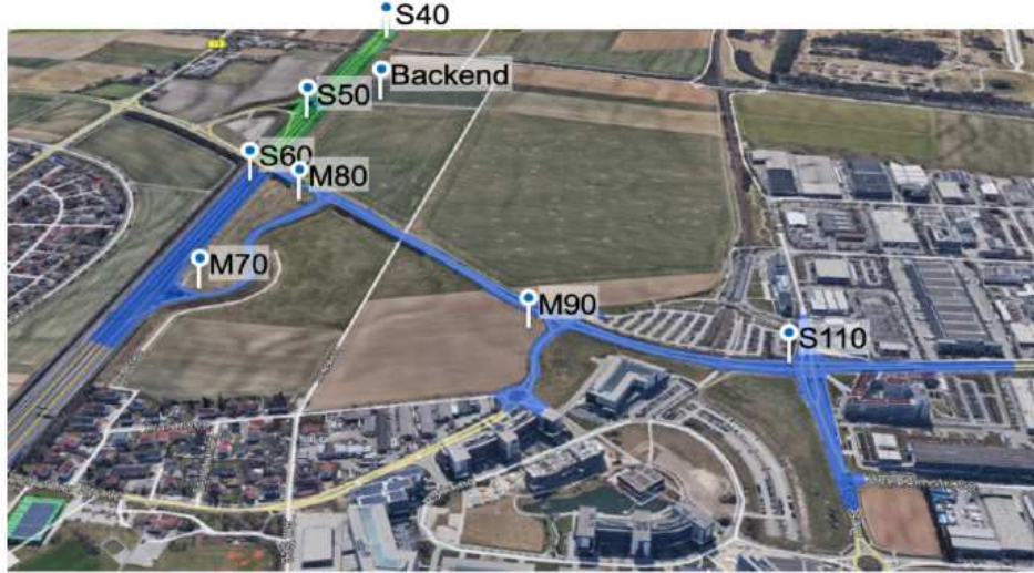
Figure 1.1: Track sections covered by the Providentia (green) and the extended Providentia++ (blue) project with marked sensor positions
