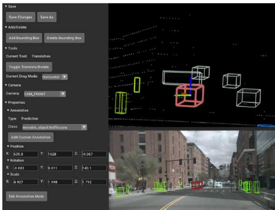
Figure 3.10: ReBound's UI shows a multi-modal view with a point cloud viewer (top) and an RGB image viewer (bottom). The editing window provides options for adding, deleting, and adjusting bounding boxes with controls for translation and rotation, as well as other properties such as the annotation type, class, and transformation parameters.
