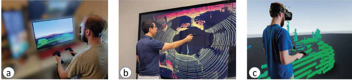
Figure 3.16: Levels of immersion: (a) An interactive non-immersive setup. (b) Semi-immersive setup. (c) Fully-immersive setup incorporating all 6 DoF.
