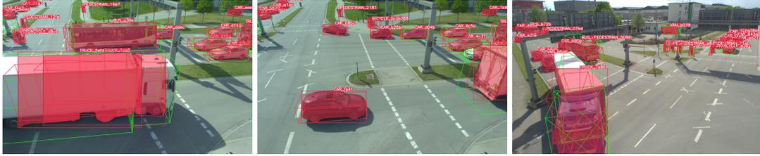
**Figure 5.2:** An Illustration comparing ground truth (green) with YOLOv8x\_tumtraf predictions (red). These frames are from the TUMTraF Intersection Dataset test sequence. The frames reveal that the labels of the TUMTraF Intersection Dataset are incomplete, failing to label all objects in the image. Consequently, the models produce false positives when identifying unlabeled objects.
